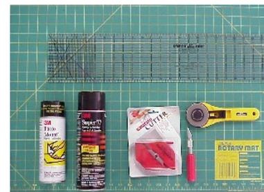
Photograph 1: Tools of the Trade: (left to right) Cans of spray adhesive for photographic paper and plain paper; both of these products were made by 3M. An exacto knife with a thick handle and a large blade gives you better control over the cut. Olfa Rotary Cutter (90 mm) and Olfa Cutting mat (35 x 23) has a useful grid for measuring. The plastic ruler is a good tool for measuring and making precise trims and makes an excellent straight edge for cutting.
